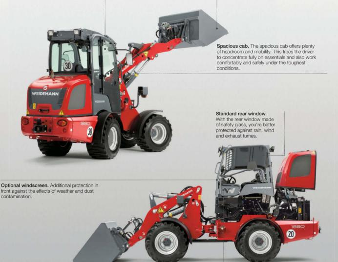
Laterally tiltable driver's cabin or cab. Easy access to the engine, hydraulic and electrical systems facilitate inspection and maintenance for you.
